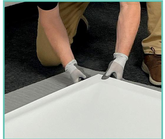
3. Tilt/stand screen upright, and continue by attaching screen surface to center points between the corners, and work from there to attach screen along the frame, joining the hook and loop strips. Gently pull and smooth screen surface while attaching it to the frame.
