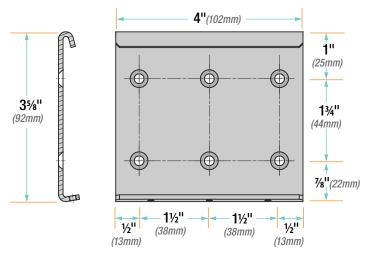
**NOTE:** Mounting brackets attach to surface with #10 Flat Head Screw.
