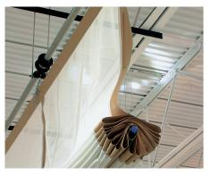
Engineered with all welded or heavy-gauge stamped hardware, the Fold-Up Gym Divider Curtains electrically divide one space into two with the turn of a key switch. The accordion fold-up action is smooth and designed for years of reliable service. Passing cables through grommets in the fabric creates an accordion fold-up action as the bottom tube is raised. Divider is available in either all solid vinyl, vinyl coated polyester mesh, or a combination of mesh on the top and solid on the bottom.
