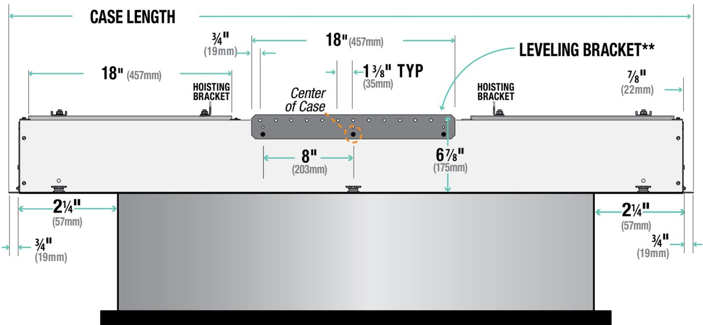
• For minimum length of ceiling cutout: subtract  $1\frac{1}{4}''$  (32mm) from case length (measured from outer edge of flanges).
